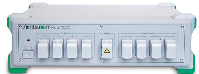
The Anritsu MT9820A characterizes optical components from 1250 nm to 1650 nm. Courtesy of Anritsu.
